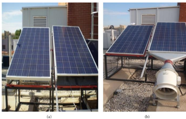
Fig. 10. Hybrid solar Photovoltaic/Thermal (PV/T) cooled by forced air circulation (a) normal solar panel (b) solar panel with forced air circulation attachment
