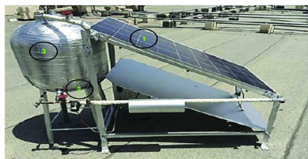
Fig. 9. Hybrid solar Photovoltaic/Thermal (PV/T) cooled by forced water circulation [28]
